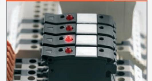
Easy identification during troubleshooting and no interference signals in control circuit – because of optional bright LED status display and minimal leakage current (less than 0.5 mA).
