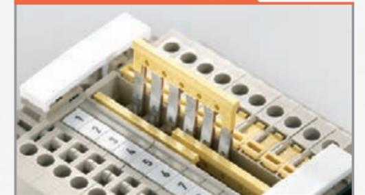
The WMF terminal block has three cross-connection channels; they are a very flexible solution for bundling and looping through of potentials. The standard ZQV cross-connections can be used to join both the neutral wire and also a shielded potential voltage across a large number of poles.
